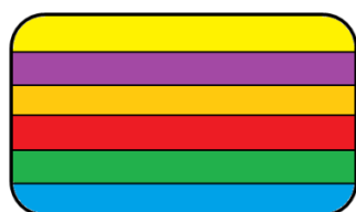
Figure 10. Cross-section of the cylinder-shaped polypill. Each color represents diverse API-containing layers: naproxen—yellow; aspirin—purple; paracetamol—orange; caffeine—red; chloramphenicol—green; and prednisolone—blue [57].
