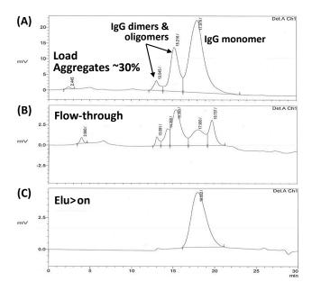
**Figure 10.** SEC-HPLC analysis of (**A**) Load on the peptide-WB column, polyclonal human IgG solution containing aggregates, (**B**) Flowthrough fraction from peptide-WB column and (**C**) Elution fraction from peptide-WB resin.
