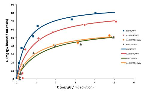
**Figure 7.** Adsorption isotherms of HWRGWV-TREN-WB, Ac-HWRGWV-TREN-WB, HWCitGWV-TREN-WB, and Ac-HWCitGWV-TREN-WB resins.
