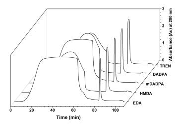
Figure 3. Breakthrough curves of the HWRGWVC-WB resins produced with different spacers.
