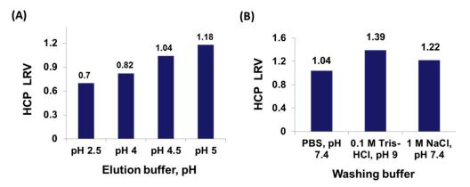
Figure 5. Values of HCP LRV obtained using different (A) elution buffers and (B) pre-elution wash buffers.
