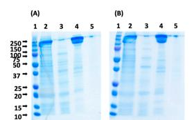
**Figure 8.** SDS-PAGE of the chromatographic fractions collected using (**A**) HWCitGWVC-TREN-WB and (**B**) Ac-HWCitGWVC-TREN-WB resins. Lanes: (1) Marker; (2) Load; (3) Flow-through; (4) Elution (pH 4.5); (5) Regeneration (pH 2.5).
