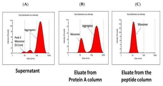
**Figure 9.** DLS analysis of **(A)** CHO cell culture supernatant, and the IgG-rich fraction eluted from **(B)** MabSelect SuRe LX and **(C)** HWRGWVC-TREN-WB resin. DLS measurements shown in Figure 9 are size distribution by intensity and therefore a small percentage of aggregates results in high peak area.
