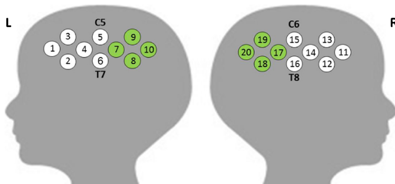
Fig. 1. Location of the NIRS channels over the left and right hemisphere, relative to 10–20 positions T7 and T8. Channels within the Region of Interest are marked green.
