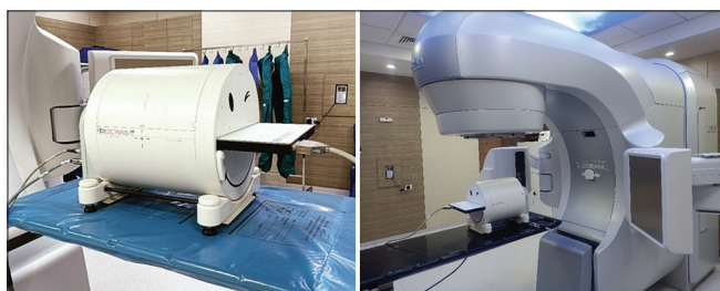
Figure 2: PTW Octavius four-dimensional phantom, TrueBeam STx LINAC
