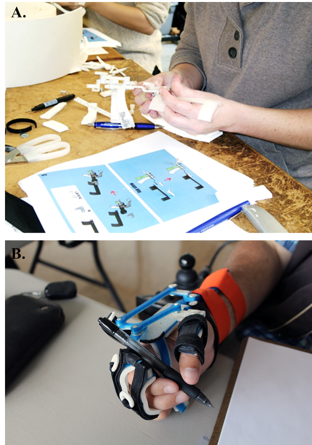
Fig 2. The experimental setup of the study with 3D-printed WDOs. (A) P&O student fabricating a 3D-printed WDO using the device manual. (B) User performs the writing task of the JTHF test with a 3D-printed WDO.
