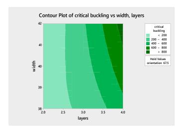
Figure 12. Contour plot of critical buckling versus width, layers.
