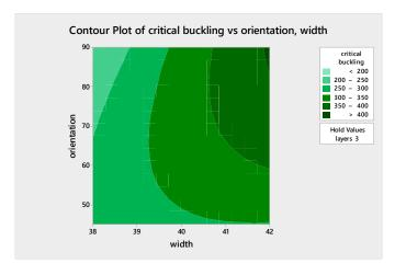
Figure 11. Contour plot of critical buckling versus orientation, width.
