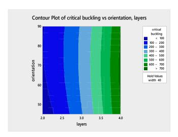
Figure 10. Contour plot of critical buckling versus orientation, layers.
