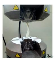
**Figure 7.** Buckling of a composite sample.
