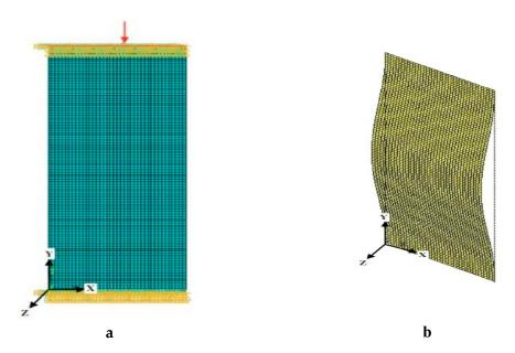
Figure 8. Meshed model (a); buckled model under a clamped-clamped end condition (b).
