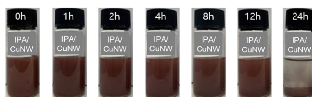
Figure 6. Dispersion stability of IPA/CuNW mixtures over time after mechanical and ultrasonic dispersion.
