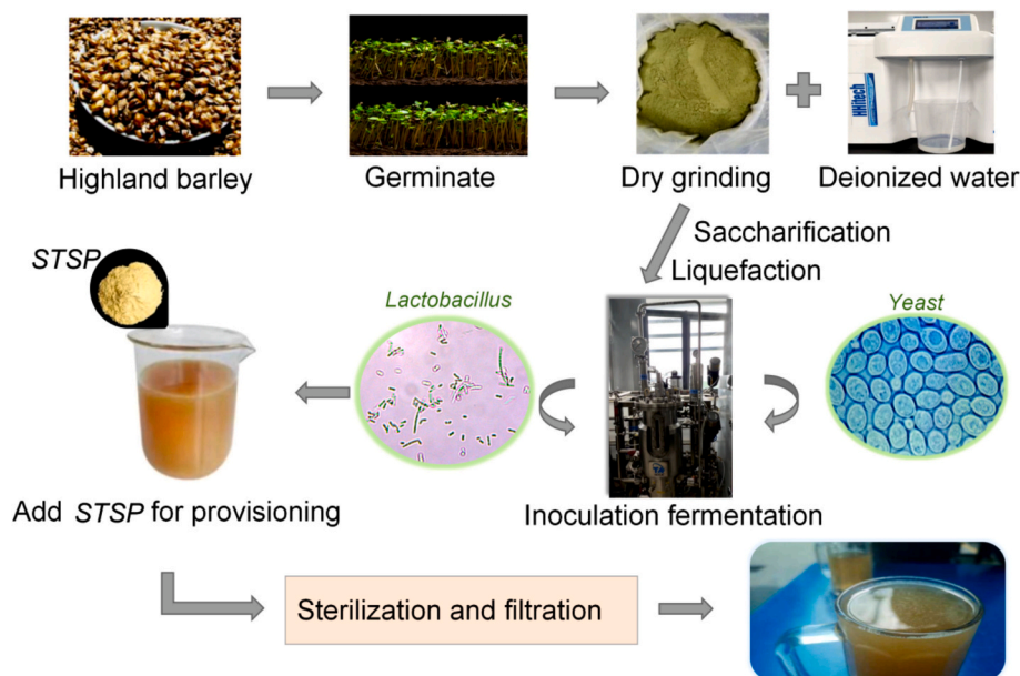
Fig. 2. The process flow diagram of beverage made by STSP compound highland barley.
