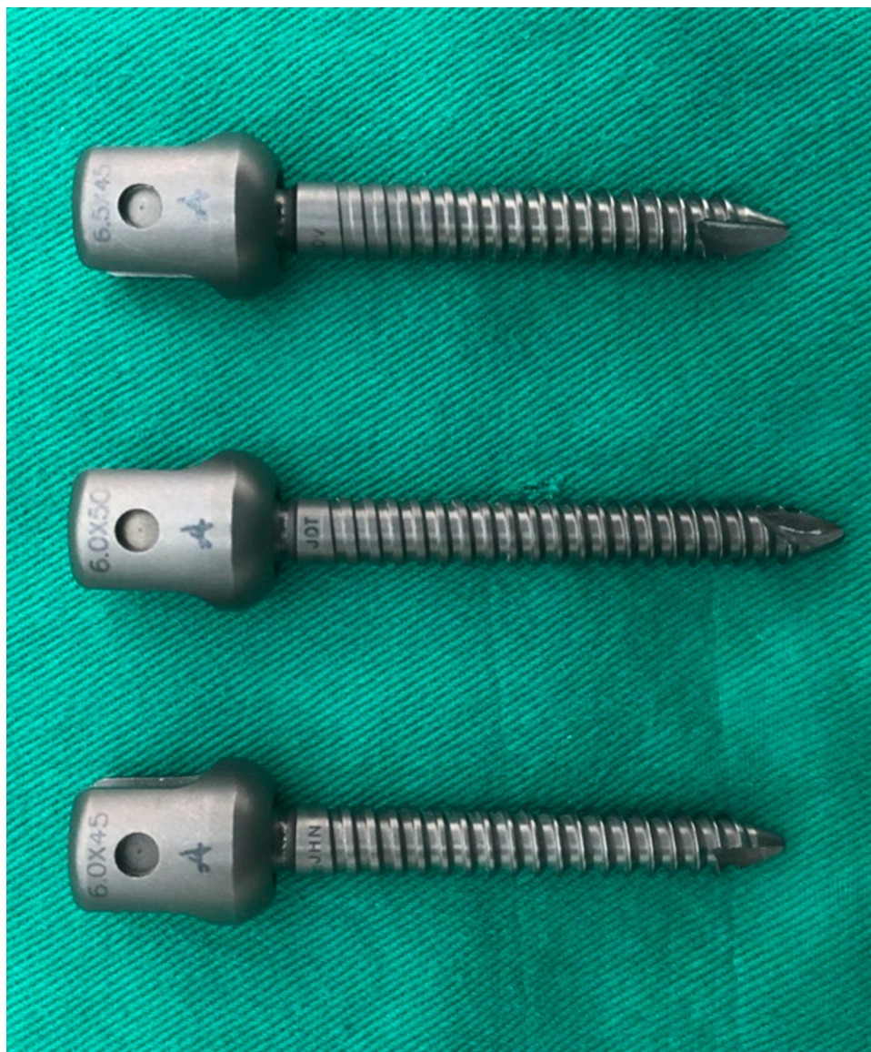
Fig 2. Photographs showing the three types of poly-axial screws used in the study. Left to right: 6.0 mm × 45 mm, 6.0 mm × 50 mm, and 6.5 mm × 45 mm (diameter × length). The length was measured from the point of the bottom of the hub to the screw tip. The diameter was defined as the outer diameter. All screw types had a thread pitch of 1 mm and a thread depth of 0.8 mm.
