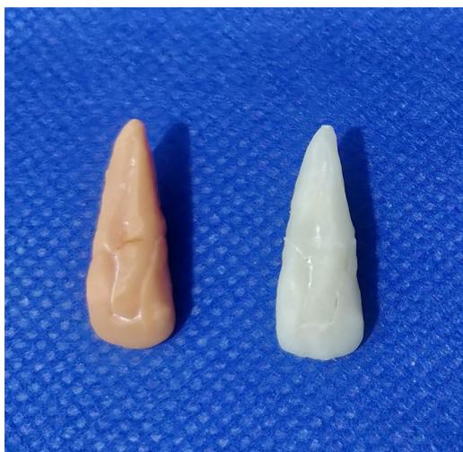
**Figure 4.** Models of reconstructed teeth which were printed using tooth printed by stereolithography (SLA) technique and tooth printed by fused deposition modelling technology (FDM) techniques (left to right, respectively).
