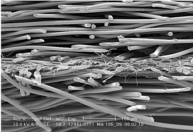
8.3 Hydroentangled composite HYCOSPUN® spunbond nonwoven with a meltblown fine fiber inside layer (used with permission from Sächsisches Textilforschungsinstitut e.V. (STFI), Chemnitz, Germany).
