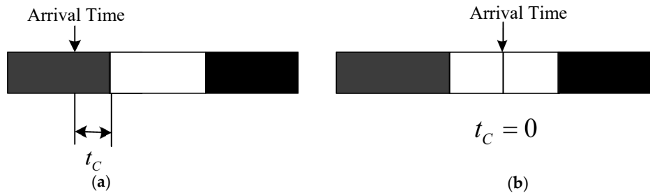
Figure 5. Schematic diagram of the waiting time and arrival time. (a) Arrive before available; (b) Arrive when available.
