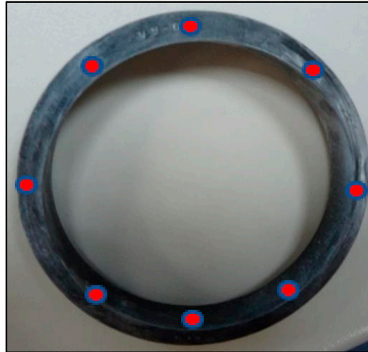
Figure 5. Front view of O-ring and position of indentations (TML).
