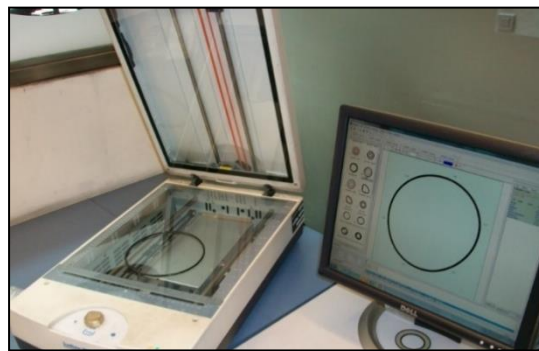
Figure 2. Dimensional checking procedure and example of measurement.
