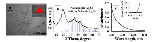
**Figure 2.** (a)—Microphotograph and particle size distribution (inset) of Ag<sub>2</sub>Se nanoparticles in AG polysaccharide matrix; (b)—diffractogram of Ag<sub>2</sub>Se-AG nanocomposite (4%w Ag<sub>2</sub>Se); (c)—absorption spectrum of 0.1% of Ag<sub>2</sub>Se-AG nanocomposite (4%w Ag<sub>2</sub>Se) water solution and its Tauc plot of  $(\alpha h\nu)^2$  vs. (hv) (inset).
