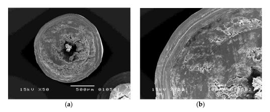
**Figure 5.** SEMs showing cross-sectional views at (a)  $50 \times$  and (b)  $150 \times$  magnification of the Ca/P/Ca/P-coated metoprolol tartrate pellets.
