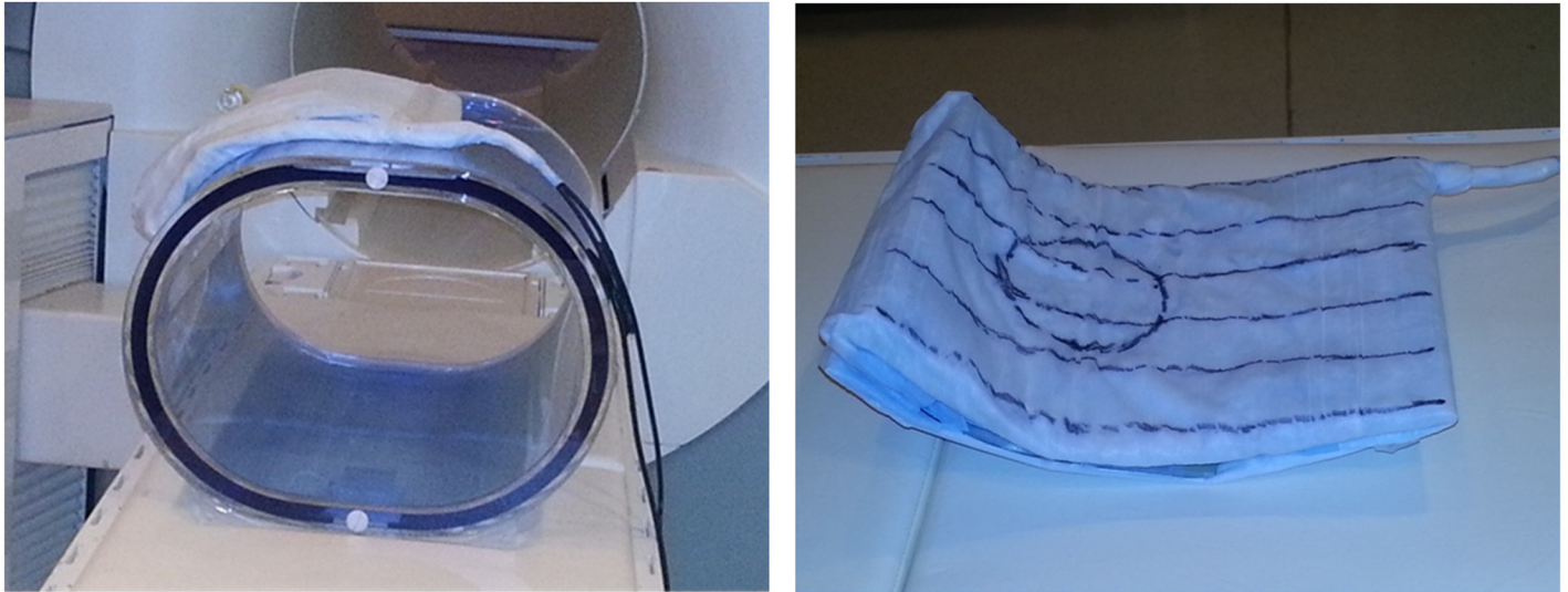
Fig 3. Photograph and layout of surface spoiling gradient coil and RF coil. The gradient/RF coil assembly was bent to contour around the torso.
