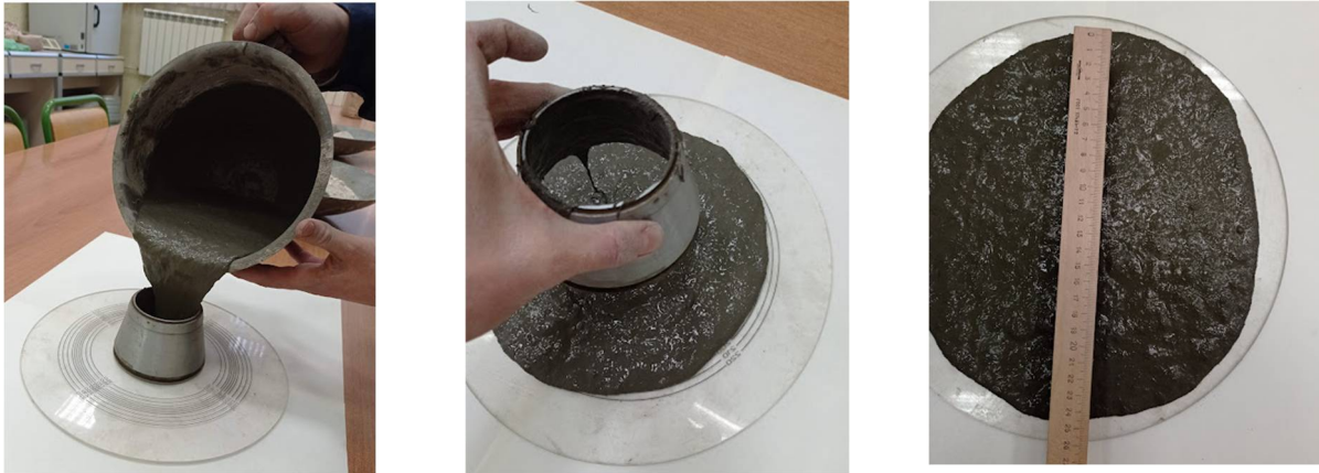
Figure 3. Workability of cement mixture with 2.5% vol. of PP microfiber.
