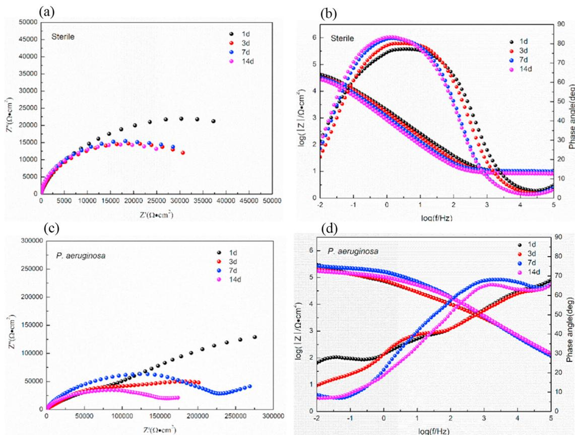
Figure 6. EIS plots of X65 steel immersed in aerobic sterile (a, b) and *P. aeruginosa* (c, d) medium for different time periods.
