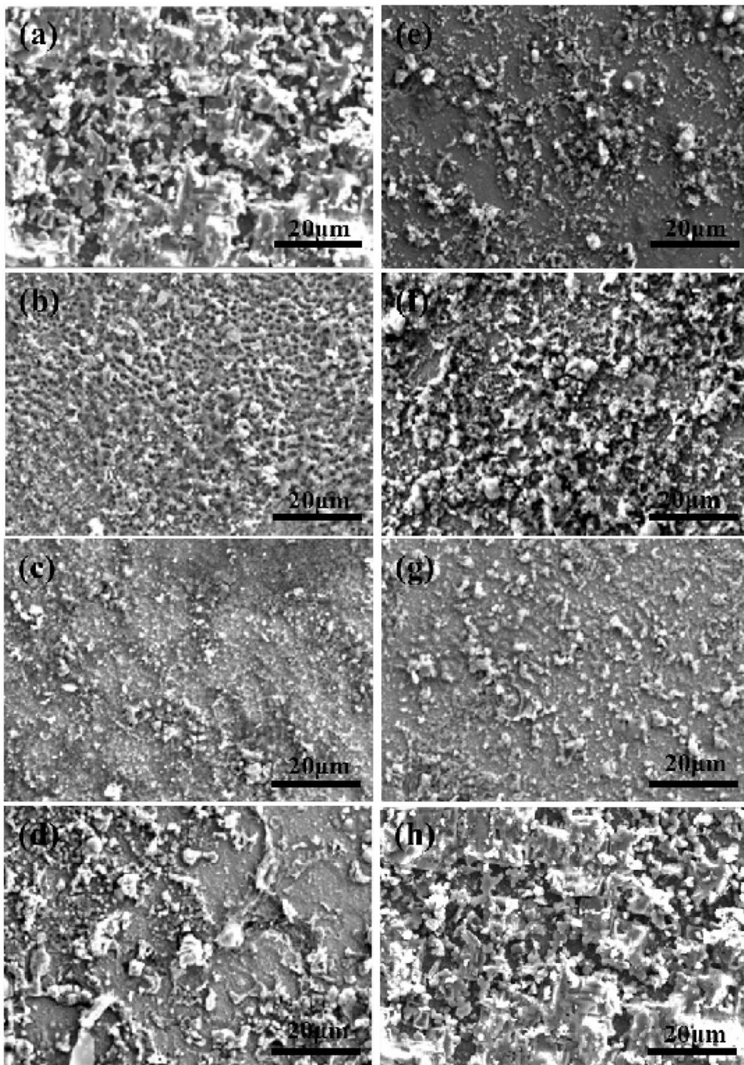
Figure 3. SEM images of X65 steel immersed in sterile anaerobic (a, b, c, d) and aerobic (e, f, g, h) conditions for 1, 3, 7, 14 days.
