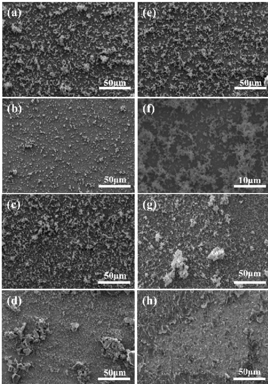
**Figure 4.** SEM images of X65 steel immersed in anaerobic (a, b, c, d) and aerobic (e, f, g, h) medium inoculated with *P. aeruginosa* for 1, 3, 7, 14 days.
