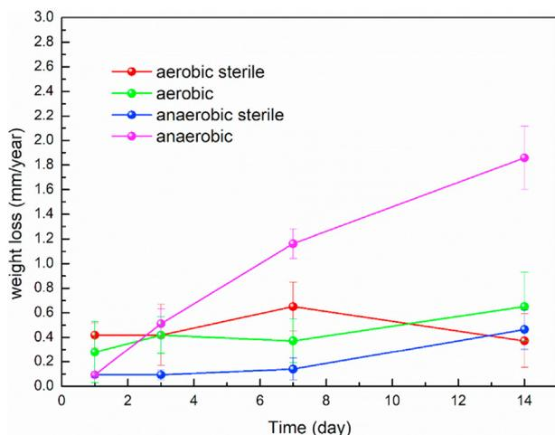
**Figure 2.** Weight loss results of X65 steel immersed in different media for 1, 3, 7 and 14 days.
