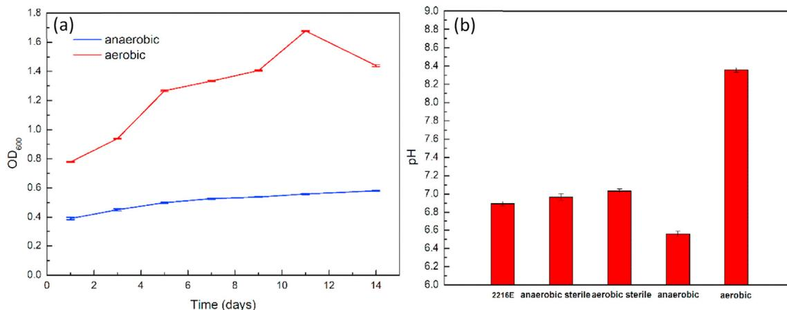
**Figure 1.** Growth curve of *P. aeruginosa* and pH value of medium with X65 steel immersed in different conditions for 14 days.
