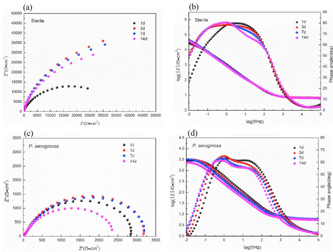
Figure 5. EIS plots of X65 steel immersed in aerobic sterile (a, b) and *P. aeruginosa* (c, d) medium for different time periods.
