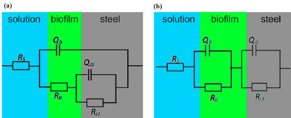
Figure 7. Electrochemical equivalent circuit used to fit EIS data.
