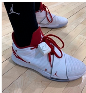
Figure 2. Positioning system (IPS) sensor placed in the protective rubber sheath on the athlete's shoelace.
