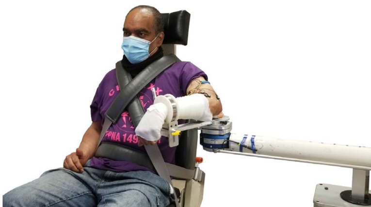
Fig. 1. Setup. Participant setup in the ACT 3D . Arm resting on lower floor at 70° abduction.
