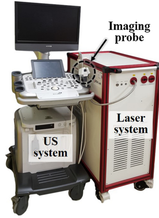
Fig. 2. Configuration and parameters of the clinical PA/US imaging system. PA, photoacoustic; and the US, ultrasound.
