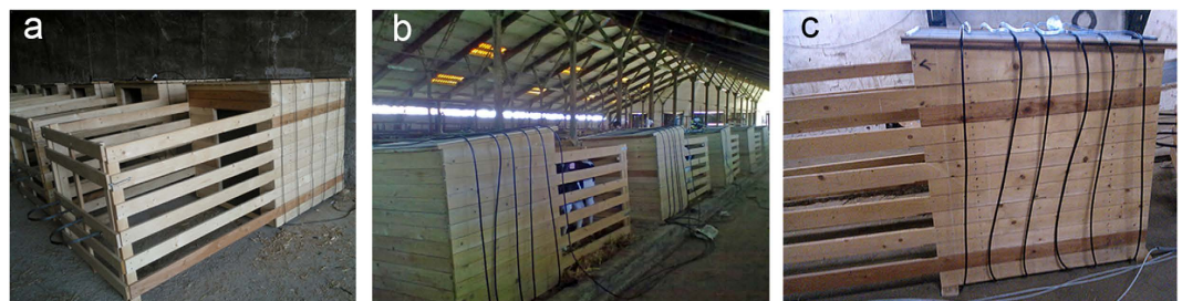
Figure 6. Individual wooden boxes for calves with coils producing ELFMF.
