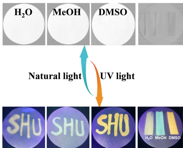
Fig. 7 The photos of the Vio1·2Cl dispersed test papers after treatment with different organic solvents under natural light and UV light.
