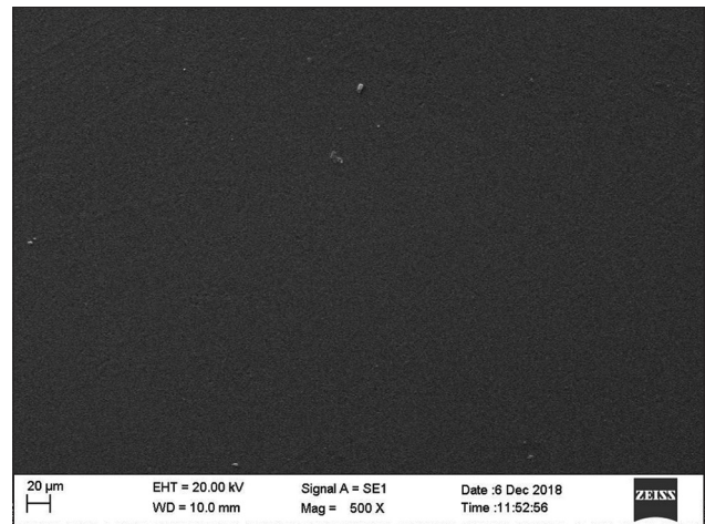
Figure 8: Monolithic zirconia roughened and autoglazed, ×500
