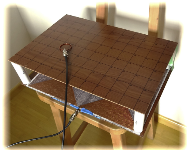
Figure 9. Experimental setup to measure the magnetic flux density generated by each coil at various distances.
