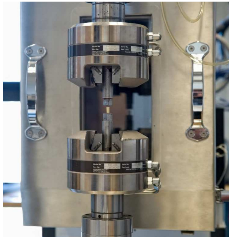
Figure 3. Testing machine grips with bone cement sample.
