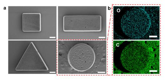
**Figure 2.** SEM–EDS images of the patterned PEGDA: (a) SEM images of the patterned PEGDA for various shapes, namely square (40×), triangle (40×), rectangular (30×), and circular (30×); (b) EDS images of circular-shaped solid drugs (scale bar: 500  $\mu$ m).
