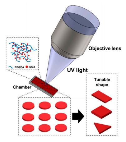
Figure 1. Schematic illustration of the proposed study: UV light is used to pattern the polymer.
