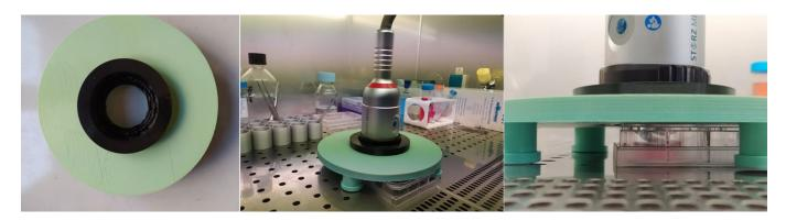
**Figure 1.** 3D-printed ESW cylindrical coil source support in PVC: the support is composed of two separate top parts (black, which adapts to the coil source size) and bottom parts (green, which keeps the support stable and suspended with respect to the 6-wellplates) were designed using Autodesk Fusion 360 (Autodesk, Inc., San Rafael, CA, USA) to minimize the loss of ESW energy at the interface between head of the device and the 6-multiwells.
