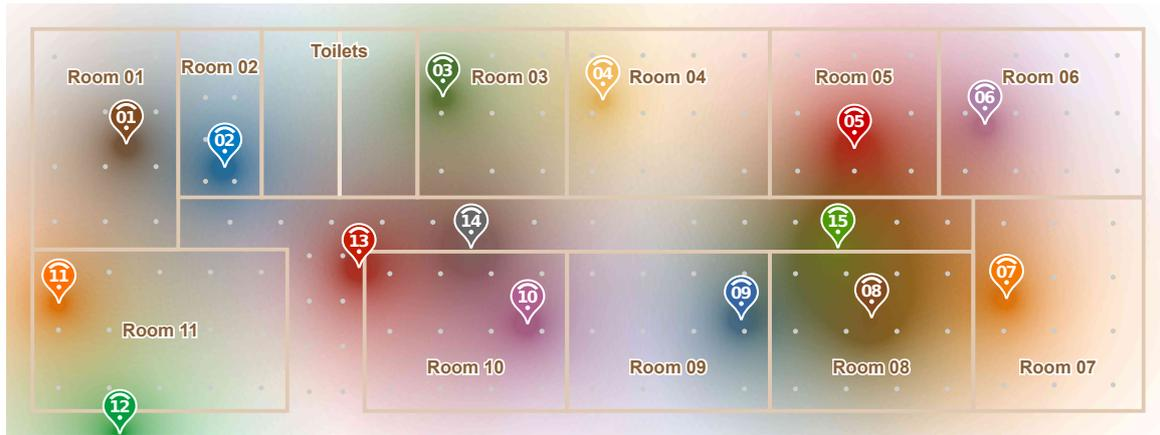
Figure 7. Signal characterization of the environment using the signal propagation model.
