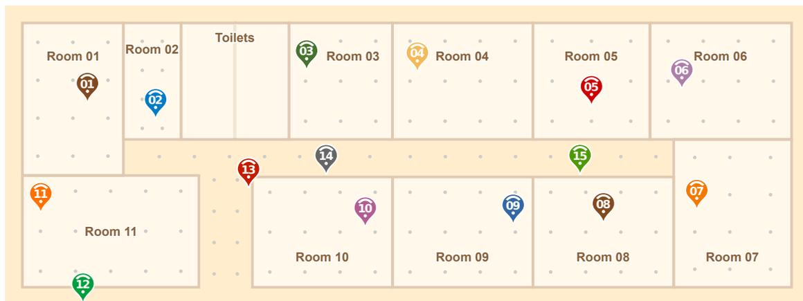
**Figure 5.** Testbed map: 11 rooms, 3 halls, and 15 anchor nodes. 100 packet samples collected from 150 test points.
