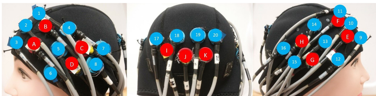
Fig. 2. The participant wore a fNIRS head cap that consisted of 11 sources (red with capital letters A-K) and 20 detectors (blue with numbers 1–20) on the scalp, distributed between the left temporal (left), occipital (center), and right temporal (right) regions. (For interpretation of the references to color in this figure legend, the reader is referred to the web version of this article.)
