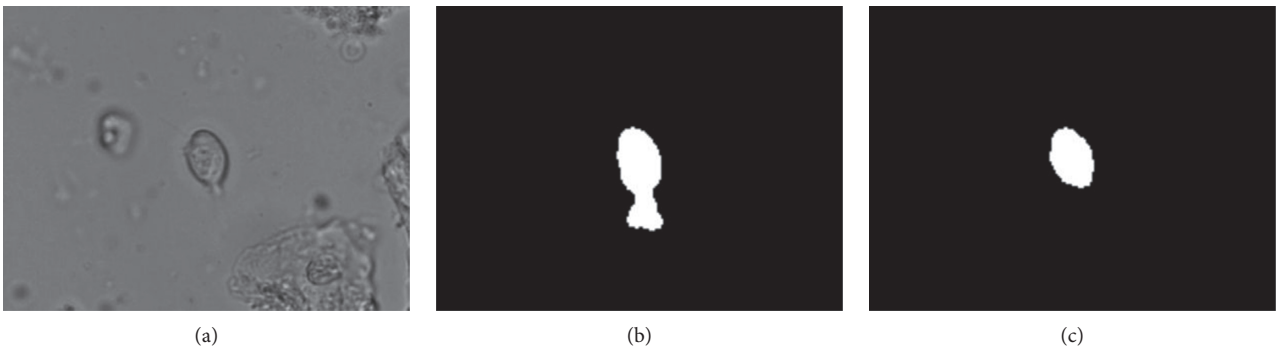
FIGURE 8: The effect of the strategy in Section 2.2.3 on eliminating the ghost region: (a) the original image; (b) K takes infinity; (c) K takes 2.
