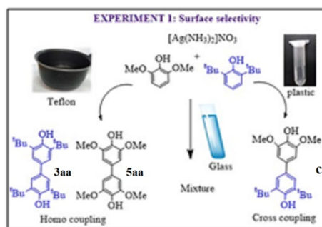
Figure 3. Two distinct Surfaces of a container directing C–C oxidative coupling between 2,6-dimethoxyphenol and 2,6-di- tert -butylphenol to major homo-coupling product (Teflon™ surface and major cross-coupling product (plastic (polypropylene and polyethylene)—Eppendorf tube). Reaction carried out in borosilicate glass tube resulted into the mixture of both these products.
