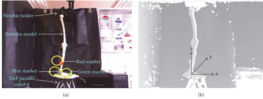
FIGURE 5: Colour marker detection by Kinect camera using KinectColorBlock software.
