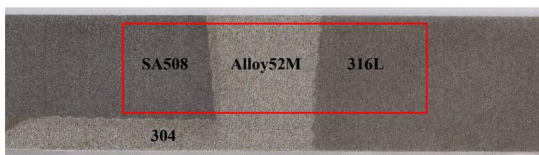
Figure 2. Physical diagram of dissimilar metal welded joints and sampling area.
