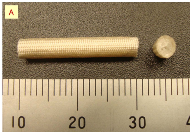
Figure 1. Polyglycolic acid (PGA) tube filled with collagen sponge (PGA-collagen tube) as a nerve guide. (A) PGA-collagen tube and its transverse section. (B) Scanning electron microscopic view of the transverse section of PGA-collagen tube.
