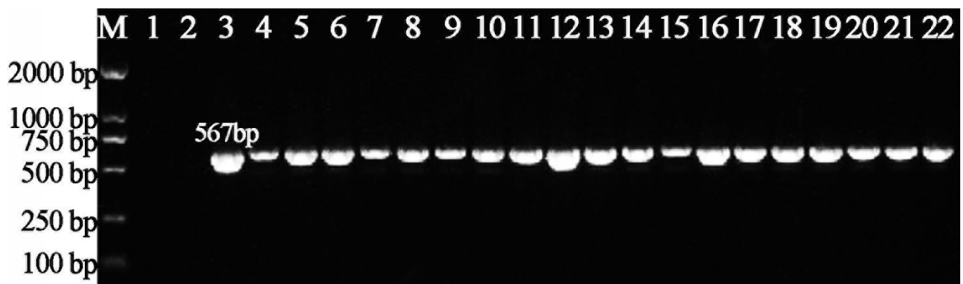
Figure 1. PCR amplification of bacteria from Tn5 mutant library according to the existence of Kan R gene on EZ-Tn5 but not in the wild type of Xanthomonas oryzae pv. oryzae strain C2. M: Maker, DL2000; 1: H 2 O; 2: WT, Wild Type; 3: positive control pRADK; 4~22: Tn5 mutants.
