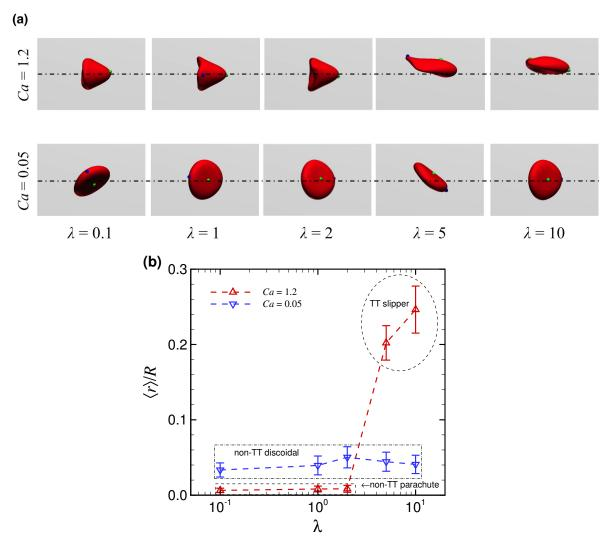
**Figure 5.** (a) Snapshots of flowing RBCs in steady state at Ca = 0.05 (bottom row) and Ca = 1.2 (top row) for different  $\lambda$ . (b) Time average of the radial position of the RBC centroid  $\langle r \rangle / R$  as a function of  $\lambda$  for Ca = 0.05 (blue inverse triangles) and Ca = 1.2 (red triangles). The results were obtained with an initial off-centered position at  $r_0 / R = 0.4$ .
