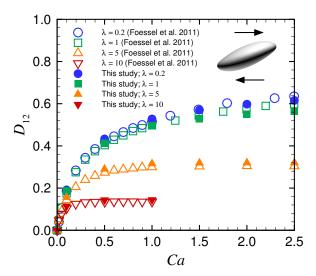
**Figure A1.** Time-averaged Taylor parameters  $D_{12}$  of an SK spherical capsule as a function of Ca for different viscosities  $\lambda$  (0.2, 1, 5, and 10); previous numerical results of Foessel et al. [48] are also displayed. The inset represents a tank-treading spherical capsule at Ca = 1.0 and  $\lambda = 1$ . The results were obtained with  $Re_p = 0.2$ .
