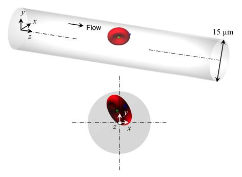
Figure 1. Simulation setup: a single RBC with radius of 4  $\mu$ m is placed with random orientation in a circular channel with diameter of 15  $\mu$ m and length of 80  $\mu$ m. Periodic boundary conditions are imposed on the flow (z-direction) and no-slip conditions are employed for the wall (x- and y-direction). Green dots represent material points at the initial concave node point, and blue dots at the initial edge node point.
