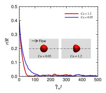
**Figure A3.** Time history of radial position of capsule centroid for different Ca (0.05 and 1.2), where the insets are the snapshots of flowing spherical capsule at steady state for each Ca (see also Videos S5 and S6). The results were obtained with Re = 0.2 and  $\lambda = 5$ .
