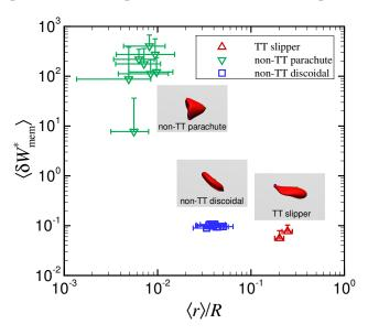
**Figure 7.** Powers associated with membrane deformations  $\langle \delta W_{mem} \rangle$  as a function of equilibrium radial position  $\langle r \rangle / R$  for different shapes. The results are replotted from Figures 4d and 6d.
