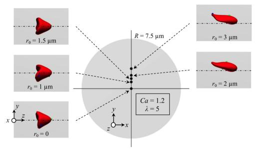
**Figure A2.** Snapshots of flowing RBCs in steady state at Ca = 1.2 for different initial positions  $r_0$  (0, 1  $\mu$ m, 1.5  $\mu$ m, 2  $\mu$ m, and 3  $\mu$ m). The results were obtained with Re = 0.2 and  $\lambda = 5$ .
