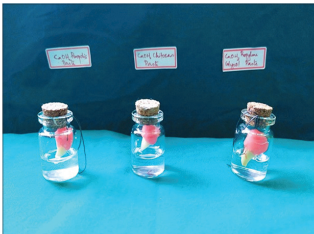
Figure 2: Each tooth from three groups with accurately measured quantities of different formulations was suspended in glass vials, such that only the apical third of the roots were immersed in deionized water
