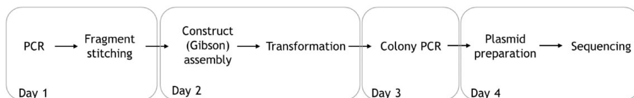
Figure 2. A simple workflow for the assembly of each part of the complete Omicron construct.
