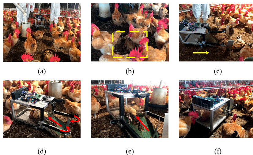
Figure 13. (a) Process of the developed system, (b) the identification of dead chickens, (c) inputting the command of the tracked vehicle, (d) inputting the commands of the conveyor belt and robot arms, (e) the movement of a dead chicken to the cache storage, and (f) the complete removal task.
