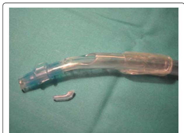
Figure 1 Amputation of the carinal hook (arrows) in a left-sided polyvinylchloride Carlens DLT (SUMI ® , Portex Inc., Mexico).
