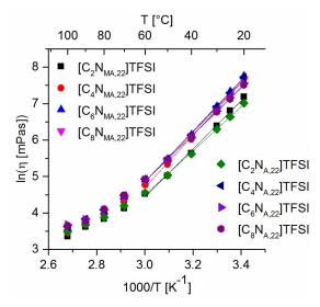
Figure 6. Arrhenius fit of viscosity values.
