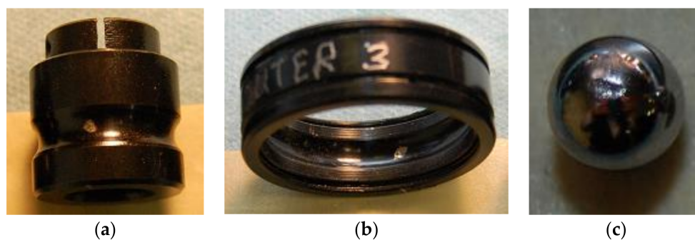
Figure 9. Physical map of three types of faults. (a) Inner race fault, (b) Outer race fault, (c) Ball fault.
