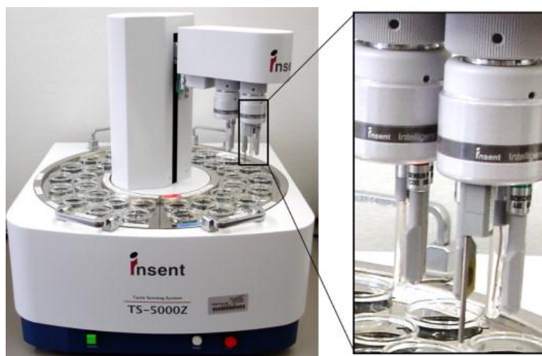
Figure 2. TS-5000Z taste sensing system, Intelligent Sensor Technology Inc., Japan. Reprinted with permission from [43] ©Elsevier).
