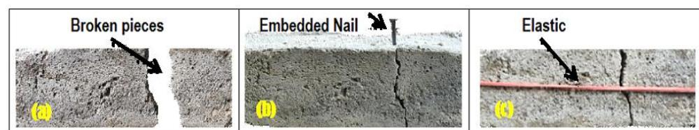
**Figure 1.** Artificial crack creation in mortar samples; (a) broken pieces; (b) Nail embedded in crack-creation setup; (c) post-crack before healing which was held using elastic.
