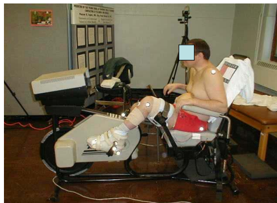
Figure 2 Complete Setup of the FES-LCE System. The subject is seated and secured within the FES-LCE system. The feet are placed in boots that are fixed to the ergometer pedal. The thighs are secured with Velcro straps, which help to maintain movement in the sagittal plane only. Seat depth is adjusted so that the subject's leg does not fully extend when the ergometer pedal is 110° with respect to TDC. Reflective markers were placed at the shoulder, hip, knee, ankle, toe, heel of boot, pedal spindle, pedal force sensor, ergometer crank center, and ergometer frame.
