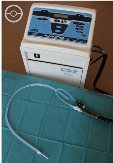
FIGURE 5: Photograph of the esophageal heat exchange device attached to the Blanketrol III temperature management unit. A cross section of the device is represented in the upper left corner.
