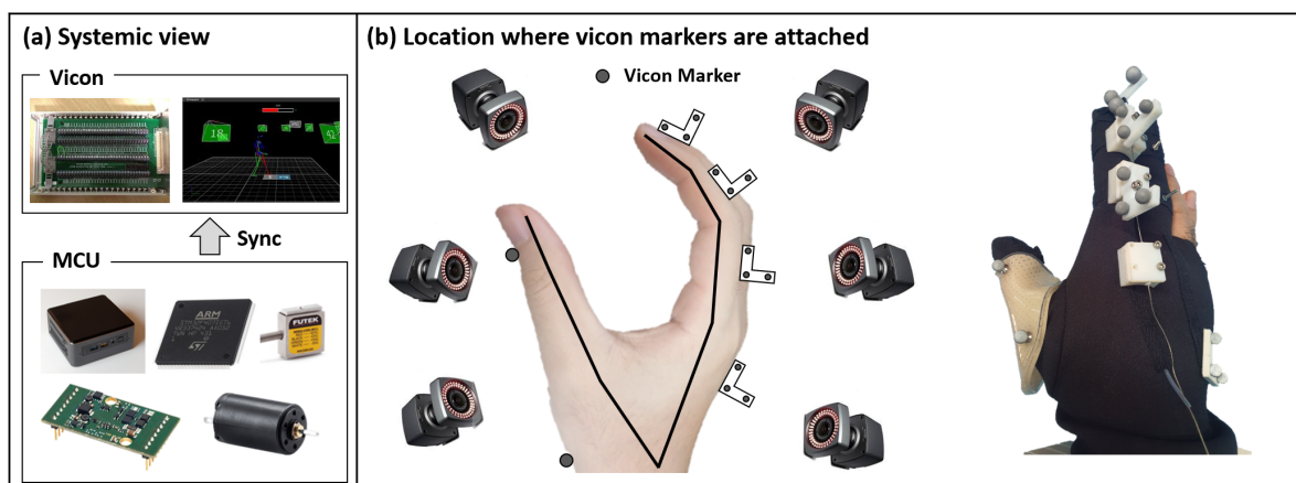
Figure 8. Schematic view of the experimental protocol: (a) shows a systemic view of vicon and the control system. By transmitting a sync signal to the ADC converter of the Vicon system, the loadcell data and encoder data were synchronized with the Vicon data. (b) shows the location where vicon markers are attached. A Total 14 markers are used in this experimental setup; 12 markers are used for the index finger and two markers are attached to the thumb to measure the thumb position.
