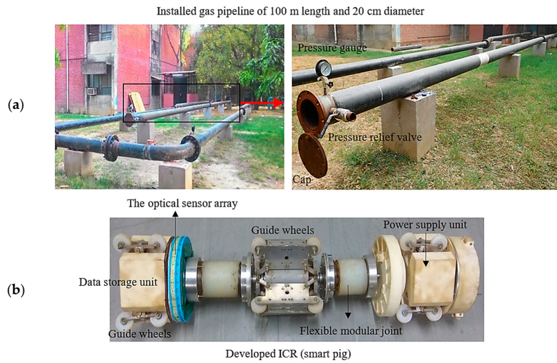
Figure 15. Images of the field test for in-line application; (a) gas transporting pipeline, (b) the designed FIG.
