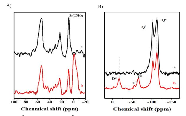
**Figure 10.** (**A**) <sup>13</sup>C MAS NMR spectra and (**B**) <sup>29</sup>Si MAS NMR spectra of (**a**) COK-5 and (**b**) IEZ-COK-5. Reprinted with permission from ref. [40]. Copyright 2015, Elsevier.
