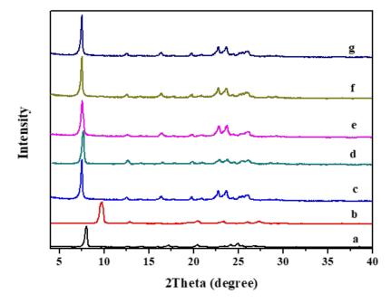
Figure 1. XRD patterns of (a) RUB-36, (b) CDO zeolite, (c) IEZ-RUB-36, (d) IEZ-CDO, (e) IEZ-Al-RUB-36, (f) Fe-IEZ-RUB-36, and (g) Fe-IEZ-Al-RUB-36. Reprinted with permission from ref. [49]. Copyright 2020, MDPI.
