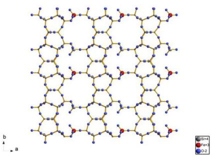
**Figure 15.** Projection along [001] of the framework of Fe-IEZ-CDO showing schematically the metal centers at every linker site. Reprinted with permission from ref. [66]. Copyright 2016, Elsevier.
