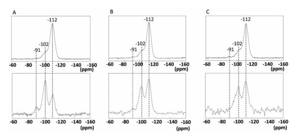
**Figure 11.** Single pulse (top) and H-CP <sup>29</sup>Si MAS NMR spectra (bottom) of (**A**) acid-only-treated RUB-36, (**B**) Fe-IEZ-CDO, and (**C**) IEZ-Al-CDO. Reprinted with permission from ref. [65]. Copyright 2014, The Royal Society of Chemistry.
