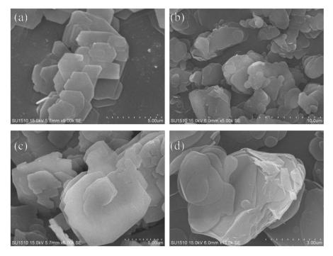
**Figure 5.** SEM images of (**a**) RUB-36, (**b**) IEZ-CDO, (**c**) Fe-IEZ-CDO and (**d**) Fe-IEZ-Al-CDO. Reprinted with permission from ref. [49]. Copyright 2020, MDPI.
