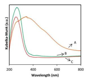
**Figure 12.** UV-vis spectra of (**A**) Fe<sub>2</sub>O<sub>3</sub>-ZSM-5, (**B**) Fe-IEZ-CDO, and (**C**) Fe-IEZ-Al-CDO. Reprinted with permission from ref. [65]. Copyright 2014, The Royal Society of Chemistry.
