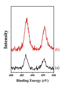
**Figure 13.** Sn  $3d_{5/2}$  and  $3d_{3/2}$  spectra of (**a**) Sn-IEZ-COK-5 and (**b**) Sn-IEZ-MFS. Reprinted with permission from ref. [55]. Copyright 2015, Elsevier.
