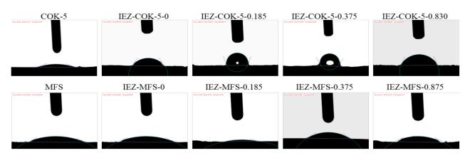
**Figure 9.** Contact angles of water on surface of COK-5, MFS, IEZ-COK-5, and IEZ-MFS produced using different amounts of DCDMS. Reprinted with permission from ref. [40]. Copyright 2015, Elsevier.
