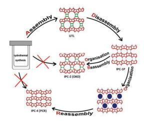
**Figure 18.** The ADOR method in a cycle scheme demonstrating the mechanism for the synthesis of two novel zeolites, IPC-2 (OKO) and IPC-4 (PCR), in which of them have not been sofa prepared by direct hydrothermal synthesis. The interlay bonds are highlighted in green, and the terminal silanol groups in blue. Reprinted with permission from ref. [8]. Copyright 2015, Royal Society of Chemistry.
