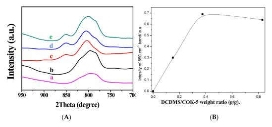
**Figure 8.** (A) IR spectra of (a) COK-5, (b) IEZ-COK-5-0, (c) IEZ-COK-5-0.185, (d) IEZ-COK-5-0.375, (e) IEZ-COK-5-0.830. (B) Intensity of 850 cm<sup>-1</sup> band as a function of the amount of DCDMS used in the silulation of COK-5. Reprinted with permission from ref. [40]. Copyright 2015, Elsevier.
