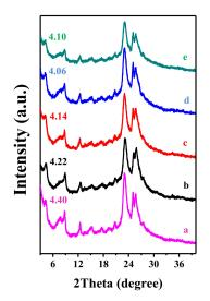
Figure 4. XRD patterns of (a) as-synthesized COK-5, (b) IEZ-COK-5-0, (c) IEZ-COK-0.185, (d) IEZ-COK-0.375, and (e) IEZ-COK-0.830. Reprinted with permission from ref. [40]. Copyright 2015, Elsevier.
