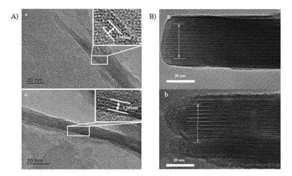
**Figure 6.** HRTEM images of (**A**)/(**a**) COK-5, (**A**)/(**b**) IEZ-MFS, (**B**)/(**a**) Ti-MWW, and (**B**)/(**b**) IEZ-Ti-MWW. Reprinted with permission from ref. [38,40]. Copyright 2004, Wiley and Copyright 2015, Elsevier.
