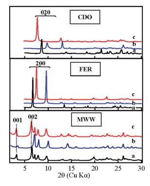
**Figure 2.** XRD patterns of (**a**) lamellar precursors, (**b**) 3D zeolites formed by the direct calcination of precursors, and (**c**) IEZs samples after further calcination. Reprinted with permission from ref. [36]. Copyright 2008, American Chemical Society.
