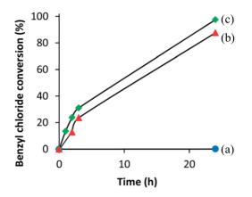
**Figure 17.** Benzyl chloride conversion in benzylation of toluene as a function of time at 403 K for (a) IEZ-Al-CDO, (b) Fe-IEZ-CDO, and (c) Fe-IEZ-Al-CDO. Reprinted with permission from ref. [65]. Copyright 2014, Royal Society of Chemistry.
