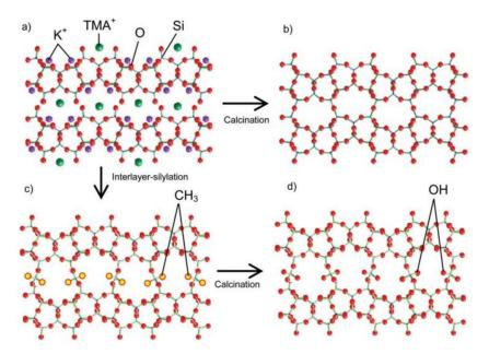
**Figure 14.** Possible schemes for the formation of the interlayer-expanded structure by the intercalation of DCDMS molecules: (a) PLS-1, (b) CDS-1, (c) IEZ-PLS-1, and (d) IEZ-CDS-1. Reprinted with permission from ref. [47]. Copyright 2007, Royal Society of Chemistry.
