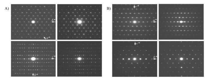
**Figure 7.** Selected-area electron diffraction patterns of (**A**) 3D MWW (left), IEZ-Ti-MWW (right) and (**B**) 3D-FER (left), IEZ-FER (right). Reprinted with permission from ref. [36]. Copyright 2008, American Chemical Society.
