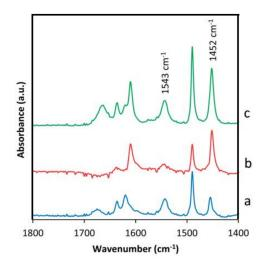
**Figure 16.** Different Py-FTIR spectra of adsorbed pyridine on (**a**) Al-CDO, (**b**) Fe-IEZ-CDO, (**c**) Fe-IEZ-Al-CDO. Reprinted with permission from ref. [65]. Copyright 2014, The Royal Society of Chemistry.
